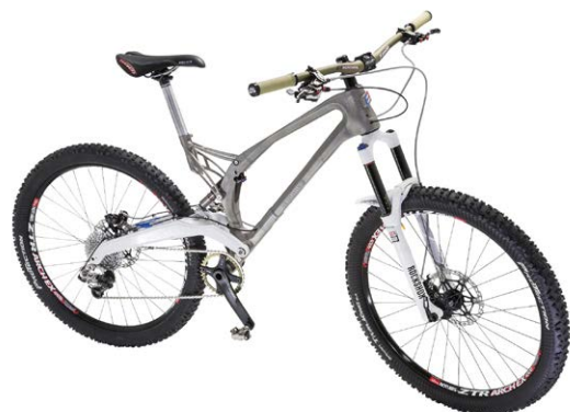
This mountain bike was developed by Renishaw and Empire Cycles using additive manufacturing
